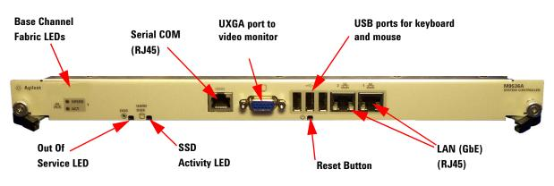
The following figure shows the front panel for the M9536A. Information about installing the controller and basic use follows in this manual.
