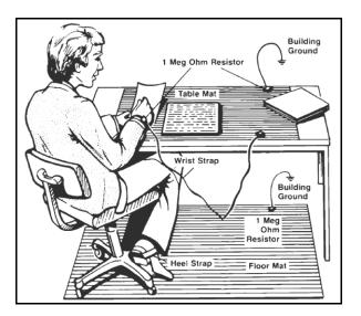
Both methods, when used together, provide a significant level of ESD protection. Of the two, only the table-mat and wrist-strap combination provides adequate ESD protection when used alone. To ensure user safety, the static-safe accessories must provide at least 1 M $\Omega$  of isolation from ground.
